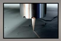
Our CNC cutting machines are designed for maximum productivity and optimal production quality. Leather defects/scars are recognized by a camera system and not processed.
